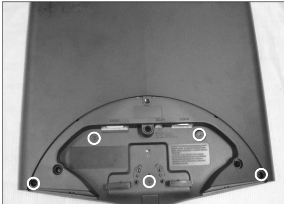
Remove the screws.
